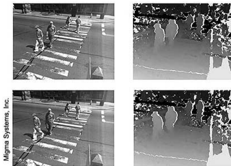
This figure shows two consecutive images (left, top and bottom), and their respective disparity maps (right, top and bottom), taken at a sampling time of 200 milliseconds.
